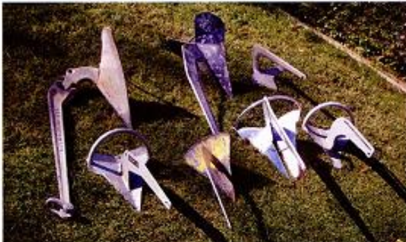
Fig. 3 - the anchors tested, from the left, back row, 22 kg CQR, 16 kg Delta, 5 kg Atlantic (Bruce copy); front row, 4 kg Rocna, 5 kg Spade, 8 kg Knox, 10 kg Manson Supreme.
